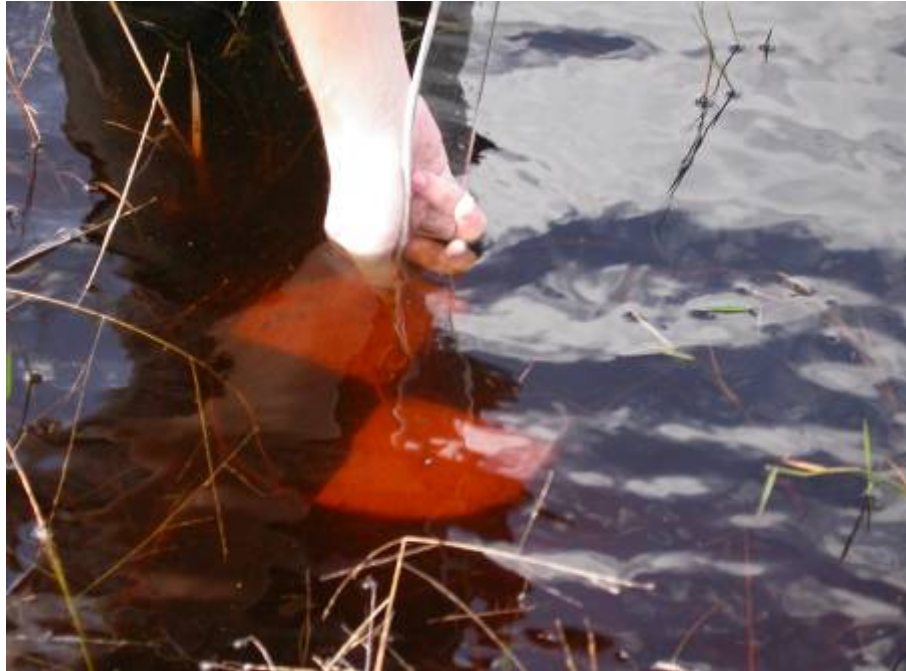
Fig. 2.2: Measuring the depth of light penetration
